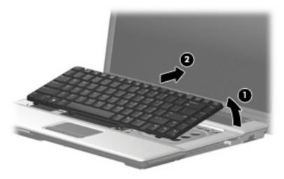
Release the zero insertion force (ZIF) connector (1) to which the keyboard cable is attached, and disconnect the keyboard cable (2) from the system board.
